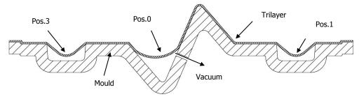
Figure 1: Indicative schematic of the inadequate drape encountered with trilayer 6
